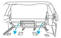
1. With assistance, lift the seat into the rear of the vehicle and position front rollers onto the track. By rolling the seat forward, guide the seat positioners over the front pins of the floor tubs.
